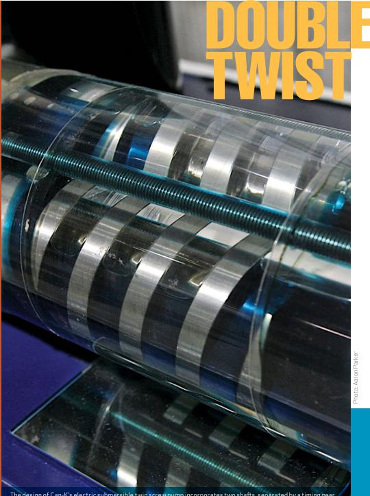
The design of Can-K's electric submersible twin screw pump incorporates two shafts, separated by a timing gear. Each shaft carries short sections of screws that interlock at extremely close tolerances but never touch. turnkey project because no other artificial lift technology can handle such a well at depths in excess of 12,500 feet deep.
