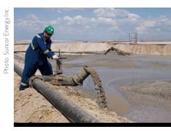
Suncor pumps a slurry of mature fine tailings and polymer flocculant over a gently tilted slope for drying. The TRO process works only during seasons without freezing weather.
